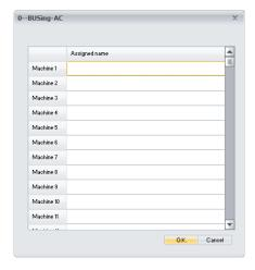
The only thing that needs to be programmed in this part, is to name the machine 1, which will be the one appearing, when linking it, on the graphical interfaces. The rest of the machines will not be used, as this gateway can only control one climate unit.
