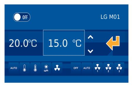
On the left side, the ambient temperature can be read, the next value in the rectangle is the setpoint temperature. Finally, at the left bottom are the available modes of the AC unit, and on the right side the speed.
