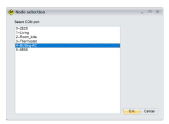
Again, a window will appear to select the Panasonic machine to add. It is reminded that this gateway only controls 1 indoor climate unit, so only the first machine should be selected, though 0 to 63 machines are available. This is because that BUSing-AC icon added in *Installation Modules* serves to program other BUSing AC gateways that can control more than one AC unit.
