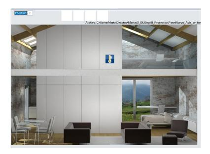
The next step will be to make a point-to-point link of the thermostat icon with the AC gateway. To do this, you must right click on the icon and select the option *Link control point-to-point*.
