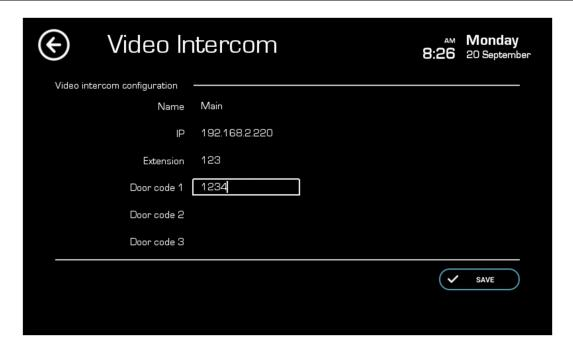
Once the data has been entered, SAVE button is pressed and we would have the VIIP configured to receive calls from the video intercom.
