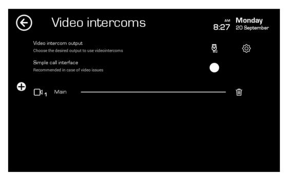
Once it is configured, you must configure the connection of the VIIP with the video intercom, click on the Video intercom output button until the icon of port 1, port 2 or Wi-Fi appears.
