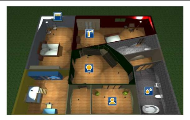
Once we have inserted the icons, we should assign the corresponding outputs of the actuator. For instance for the light icon we will assign output 1 (one light) of the KI1 by pressing on the right button of the mouse on the icon and selecting "edit properties".
