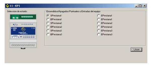
Click on "Close". The node and the corresponding output of KP1 are assigned to the blind icon.
