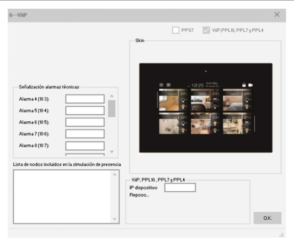
Make sure that the screen has only one IP address and the Wi-Fi net is working properly. If the device has been previously configured, we will only need to introduce the IP of the device and click on "Program".
