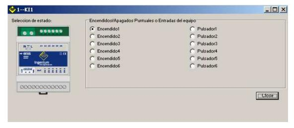
Click on "Close" and the icon will be assigned to the control of this output. If you put the mouse on the icon you will get the information about the assigned node and output. This information is shown on the left upper part of the screen. In this case it is Node 1 (KI1, because in the example it is in address 1) and output 0 (because "Light 1" is output 0).
