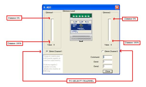
There are two dimmer channels: Dimm Channel1 and Dimm Channel2. Each one has two vertical slide bars where you select the load power percentage value (i.e., greater or less light supplied to lightbulbs connected to each dimmer channel).
