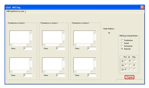
Then wait for the bar under the Program button to reach the end and you will have uploaded the data.
