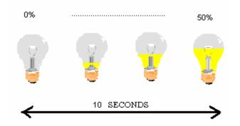
In other words, when you activate this switch, the light increases from 0 to 50% in 10 seconds.
