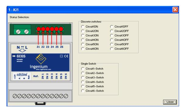
$\underline{\text{NB}}$ : Outputs Z1 to Z6 correspond exactly to the arrows shown in the image above.
