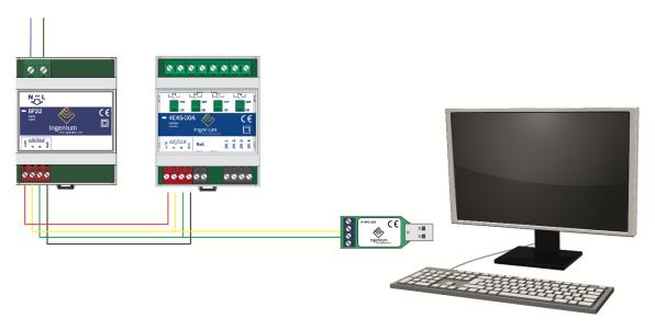
**NOTE:**IT IS NOT NECESSARY TO PLACE THE POWER SUPPLY IF THERE IS SUFFICIENT VOLTAGE IN THE INSTALLATION TO FEED IT. IT MAY BE THAT THE FEED COMES FROM OTHER DEVICE SUCH AS 6E6S, 4E4S... ETC.
