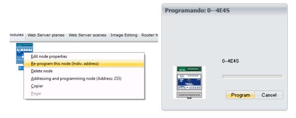
Wait until the bar on top Program button reach the end so the device has the data downloaded.
