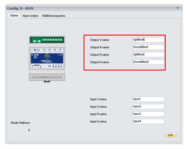
It is not normally possible to assign names to the inputs, only to the outputs in order to identify in the programming which output controls which lighting.
