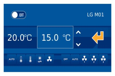
On the left side, the ambient temperature can be read, the next value in the rectangle is the setpoint temperature. Finally, at the left bottom are the available modes of the AC unit, and on the right side the speed.
