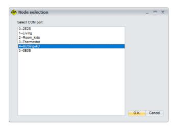
Again, a window will appear to select the Mitsubishi machine to add. It is reminded that this gateway only controls 1 indoor climate unit, so only the first machine should be selected, though 0 to 63 machines are available. This is because that BUSing-AC icon added in *Installation Modules* serves to program other BUSing AC gateways that can control more than one AC unit.
