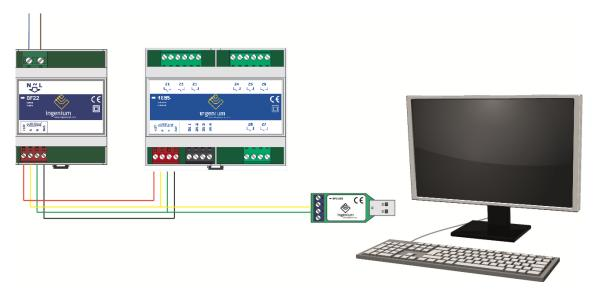
**NOTE:**IT IS NOT NECESSARY TO PLACE THE POWER SUPPLY IF THERE IS SUFFICIENT VOLTAGE IN THE INSTALLATION TO FEED IT. IT MAY BE THAT THE FEED COMES FROM OTHER DEVICE SUCH AS 6E6S, 4E8S... ETC.
