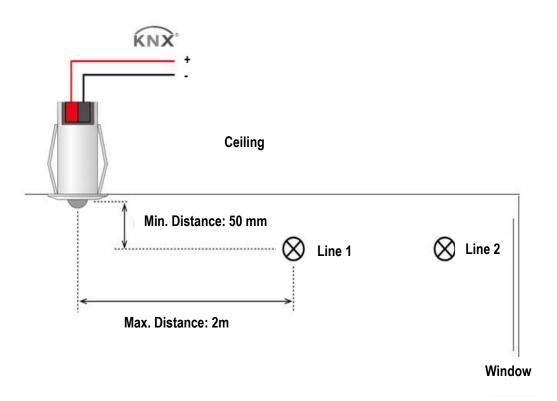
Focus the sensor for brightness measurement:
