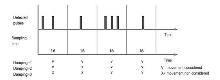
Any movement which generates an amount of pulses higher than the damping factor, during a sampling time, is considered "movement detection" by the sensor. For the same sampling time, increasing the damping, the movement should be faster and wider to generate a detection as the need of more pulses. Furthermore, a lower damping allows shorter and slower movements to be detected as well.
