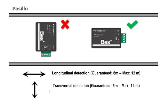
The detection area (placing the SR570000 at 2.5m from the floor) is:
