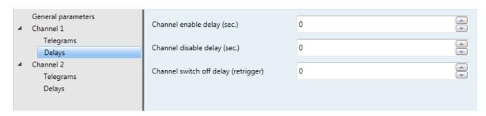
These parameters allow to configure time delays when enabling or disabling the sensor and the time that the light is on when the sensor is programmed for lightning control.
